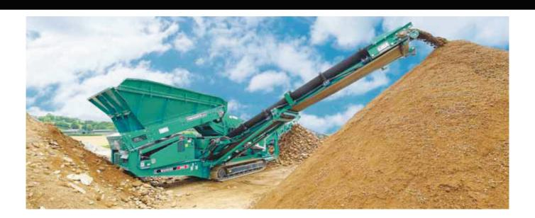
The Powerscreen® Warrior 800 has been specifically designed for the small end user for whom versatility and transportability are of key importance. The machine is a multi-purpose heavy duty incline 2 deck screen, capable of stockpiling, 3 way splitting or scalping before and after crushing units. Its highly aggressive screen can accept bofor bars, finger screens, woven mesh and punch plates.
