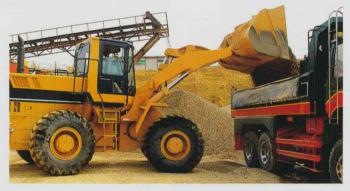
High dumping clearance, long dumping reach and excellent visibility enable easy loading of dump trucks. A center pin-supported rear axle with a  $\pm$  13° oscillation range, extra-long wheelbase, wide tread and a 40° articulation angle assure stability over the roughest terrain.
