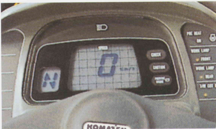
The main monitor keeps the operator constantly informed of the various travelling functions.
