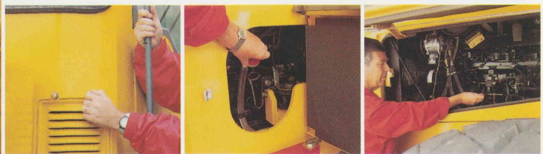
Easily accessible service points from the ground for cab filter, engine and transmission make service work simple and clean.
