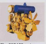
The S6D105 turbocharged diesel engine delivers 150 HP (112 kW). At the same time, the six cylinder, watercooled, direct injected diesel engine is fuel efficient, decreasing fuel consumption per hour of production. The full powershift, countershaft type transmission is suited for all jobsite conditions.
