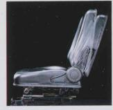
The oil-suspension seat (optional) is fully adjustable for maximum operator comfort.
