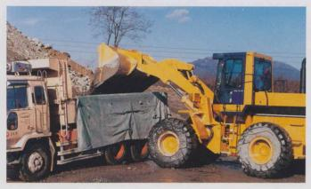
High dumping clearance, long dumping reach and excellent visibility enable easy loading of the dump truck.
