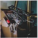
The adjustable steering wheel tilts within a 100 mm (4'') range for operator convenience.
