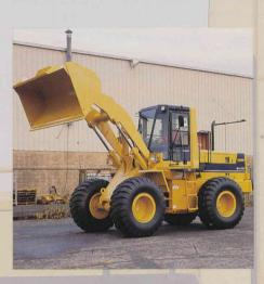
Rugged Construction – is provided by a four plate loader tower and solid plate lift arms. Coupler System – a versatile optional coupler system provides fast, efficient tool changes without leaving the cab. An optional third spool valve is available for additional hydraulic functions.
