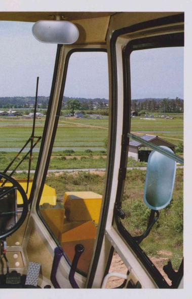
Work equipment levers are the direct control type which has good fine control performance. Little operating effort makes a comfortable operation possible.
