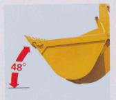
The large bucket penetrating force is properly balanced with the WA250-1's weight and drawbar pull for powerful excavation. The bucket's 48° roll back angle assures full buckets and prevents spillage of material.
