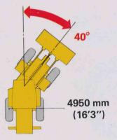
A long wheelbase with a 40° articulation on both sides enables sharp maneuvering even in limited work spaces.
