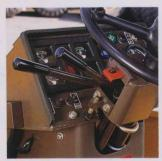
The speed and directional levers require only slight finger movements while the priority valve steering system guarantees smooth, constant steering.
