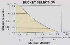
1,2 m<sup>3</sup> (1.6 cu,yd) Loose material bucket with bolt-on cutting edge (Loading and excavating soil, sand and a variety of other commonly handled materials.)
