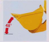
The large bucket penetrating force is properly balanced with the WA100-1's weight and drawbar pull for powerful excavation. The bucket's 48° roll back angle assures full buckets and prevents spillage of material.
