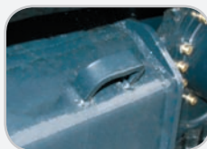
Fixing points on track frame and blade to facilitate transportation on trailers
