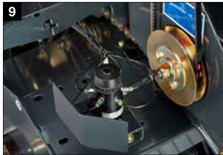
BEKA-MAX continuous chain oiling system
