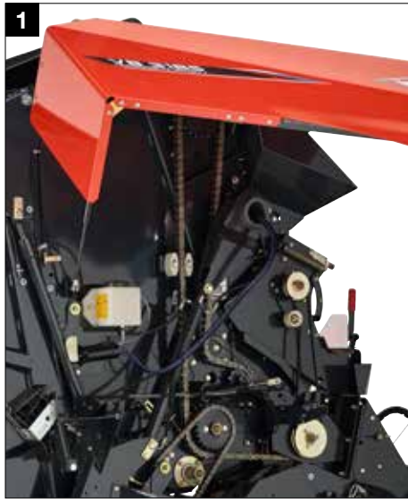
Robust driveline with high quality IWIS chains
