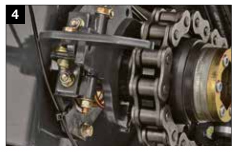
Mechanical rotor disengagement
