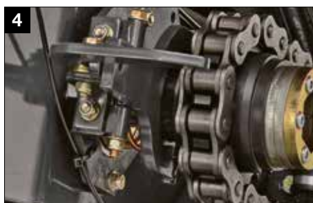
Mechanical rotor disengagement
