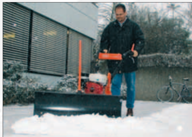
Lateral adjustment of the snow shield from the handle. Well dimensioned AG tyres as standard, lawn tyres with snow chains optionally available.
