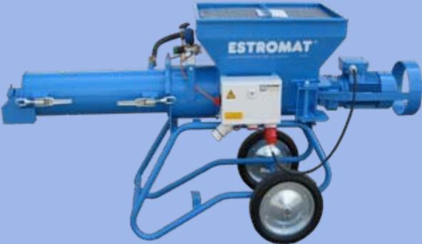
*The continuous mixer processes dry premixed material out of silos up to a grain size of 8mm, as cement-floor screed, plaster and brick-mortars, rough coat, light wall mortars, self levelling floor screed ect. Mixing capacity 40 – 120 l/min according to the dosage shaft. Silo-flange ID 250mm. Mixing tubes in various length for individual mixing time.*
