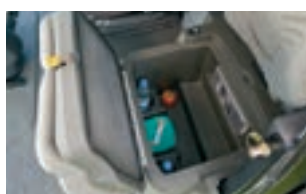
Refrigerator box integrated in trainee's seat
