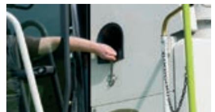
Changing the MULTICROP pre-separation concaves
