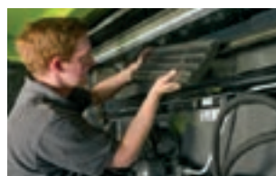
Changing the MULTICROP pre-separation concaves
