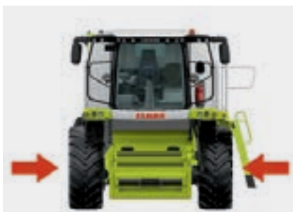
Reduced transport width with increased contact area
