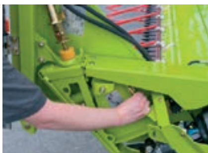
The dividers and rapeseed knives can be secured without the need for tools
