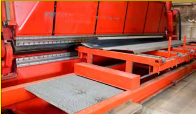
Press brake with digital control and 600 t pressure power
