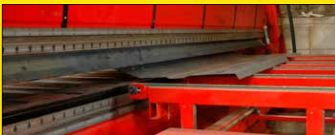
Press brake with digital control
