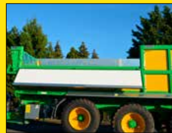
Folding side with hydraulic control
