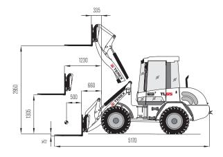
Operating load over total lift range: 1550 (1650\*) kg Operating load in transport position: 1900\* kg "With rear axle weights 3870
