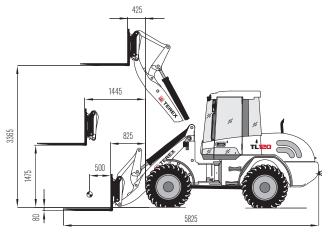
Operating load over total lift range: 2700 (3000\*) kg Operating load in transport position: 3500 kg "With rear axle weights
