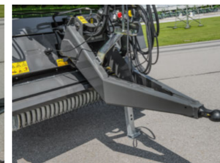
The Fendt Tigo models can optionally be equipped with a bottom hitch with ball hitch K80.
