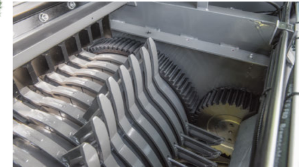
The power of the main drive is transmitted from the drive train to the rotor via extra strong spur gears with a force-locking involute gear.
