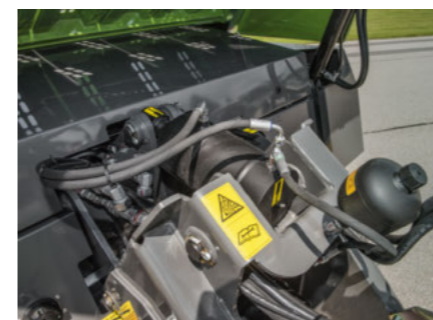
The articulated drawbar suspension reduces all shocks felt by the machines, therefore ensuring a pleasant ride.
