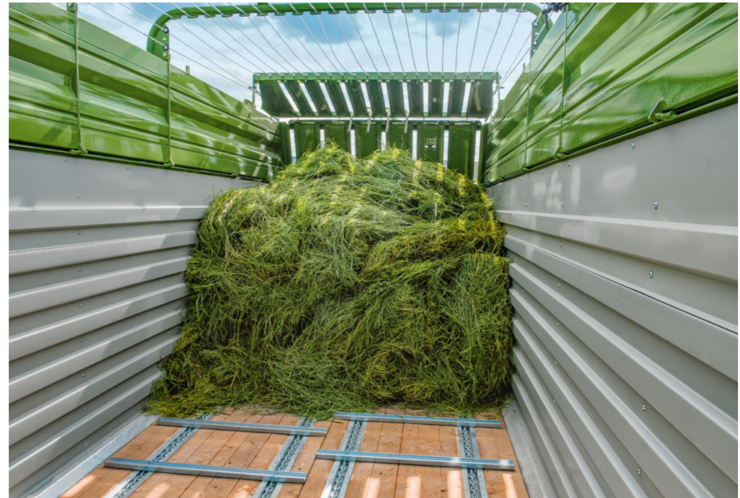
With the two-stage automatic loading system, light pressure is applied via a bar, while moderate pressure is applied via the loading flap.
