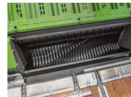
The rotor with a diameter of 800 mm and six spiral rows of teeth made of Hardox steel is equipped on both sides with large spherical roller bearings.
