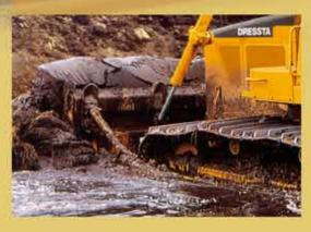
Straight blade of 3.6 cu.m (4.7 cu.yd) used with 2.16 m (85 in) gauge and 940 mm (37 in) track shoes (LGP) is designed for soft, swampy areas. This blade may be equipped with hydraulic tilt cylinder to perform efficiently landscaping operations.
