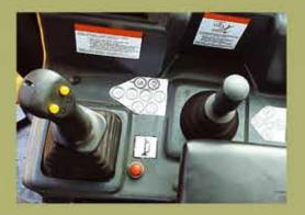
Various blade control levers are used for distinct work equipment specifications (tilt only, tilt/pitch or 6-way blade). Pilot operated hydraulic controls are offered as an option. The right hand ergonomical lever controls raise and lower of the ripper.
