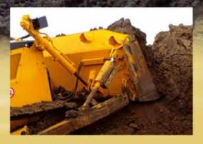
Semi-U blades of 5.7 cu.m (7.45 cu.yd) for STD & LT track frame and 5.95 cu.m (7.8 cu.yd) for WT version, combine penetration ability of straight blade with increased capacity provided by short wings.
