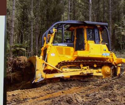
Optional sweeps and screening package are designed to provide operator protection in various types of forestry applications.
