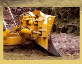
6-way hydraulic angle blade of 3.8 cu.m (5 cu.yd) used with 2.03 m (80 in) gauge wide track (WT) and max. shoe width of 560 mm (22 in) is applicable for versatile operations such as finish grading, spreading material and light land clearing.
