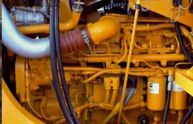
Cummins QSC8.3 engine meets U.S. EPA Tier 3 and EU Stage IIIA emissions standards. The QSC advanced electronics provide enhanced engine performance with higher torque and better throttle response at every rpm. With its ideal combination of electronic controls and durable block design, this engine is ready to meet even toughest machine work conditions.
