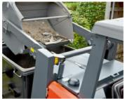
Hydraulic dirt hopper lifting system: The dirt hopper allows high dumping at heights of up to 152 cm.
