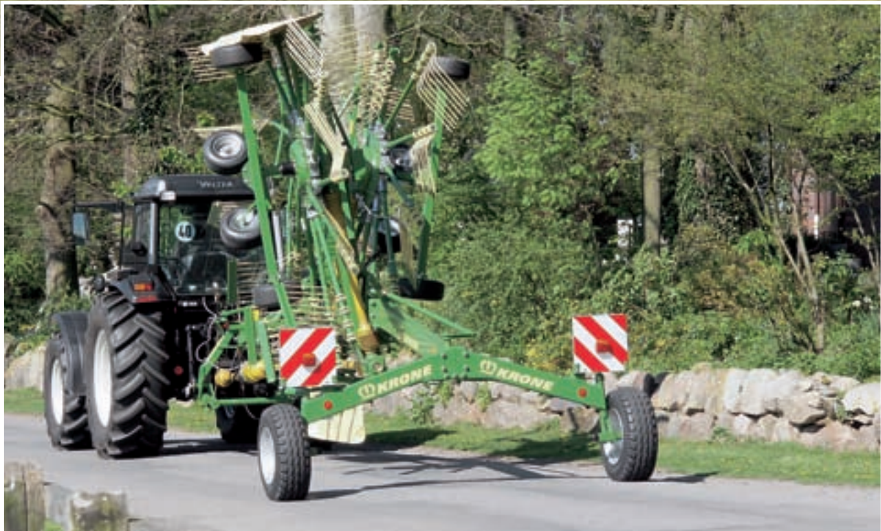
Down the road at 40 km/h (25 mph), compact and safe: when on public roads and driving underneath low bridges and underpasses, utility lines and masts the upper, outer tine arms can be folded in.
