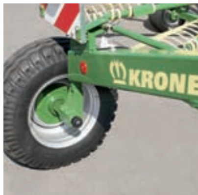
Optimally equipped: the large 10.0/75-15.3 8 PR tires and track-following linkage ensure absolutely smooth and stable travelling – an advantage when working on slopes or at high driving speeds.
