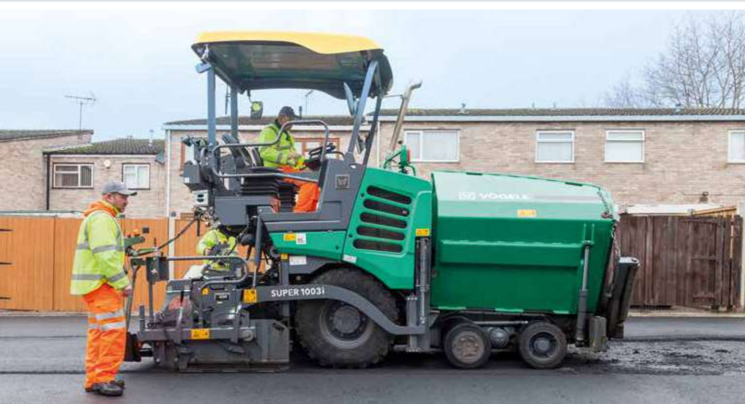
The power unit of the SUPER 1003i with diesel oxidation catalyst (DOC) and diesel particulate filter (DPF) for exhaust gas after-treatment complies with the strict requirements of European exhaust emissions standard Stage V and US EPA Tier 4f.
