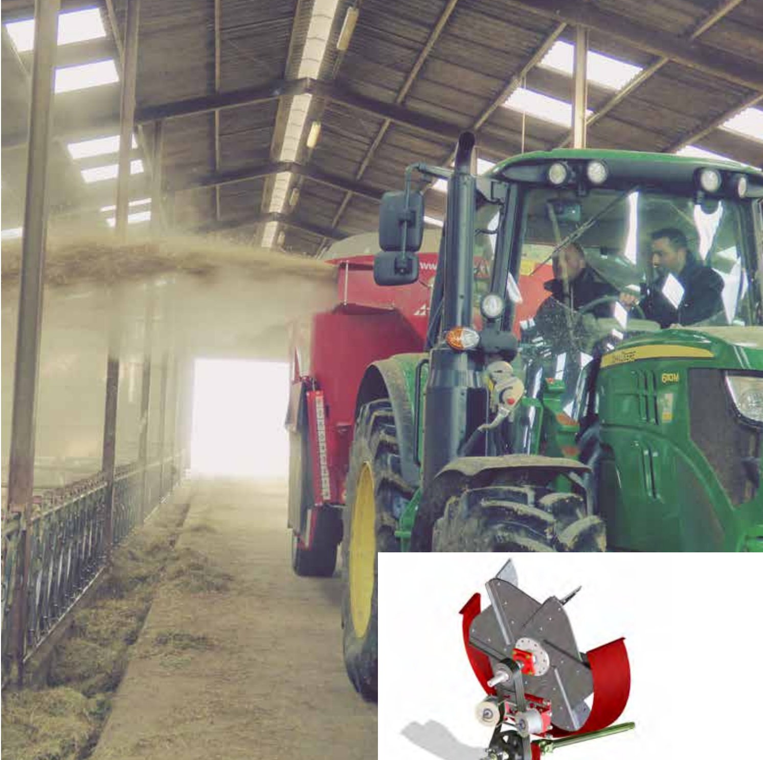
Mechanical drive with multiple drive belts so that PTO does not have to be switched on and off.
