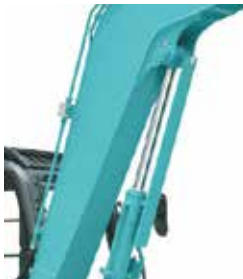
Boom: Guard plate for boom cylinder
