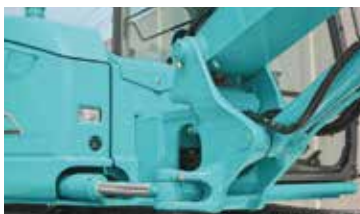
Swing bracket: Large, thick cast-iron swing bracket
