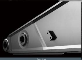
Thickness of steel plate has been increased in preference to adding reinforcing plates.
