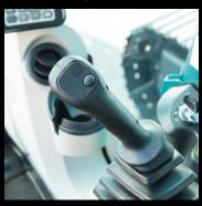
Pilot controlled joysticks have 25% lower lever effort\*, which reduces fatigue over long working hours or continued operations.
