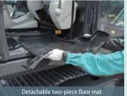
Special crawler frame design is easily cleaned Detachable two-piece floor mat with handles Engine oil pan equipped with drain valve. for easy removal. A floor drain is located under floor mat.
