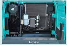
Laid out for easy access to radiator and cooling system elements
