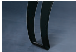
Optimized jaw shape for grapping logs
