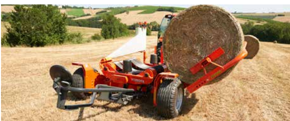
The short lifting height provides fast transfer of bale from arm to turntable.
