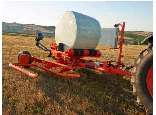
Turntable with two driven rollers designed for a high bale stability and smooth even rotation.
