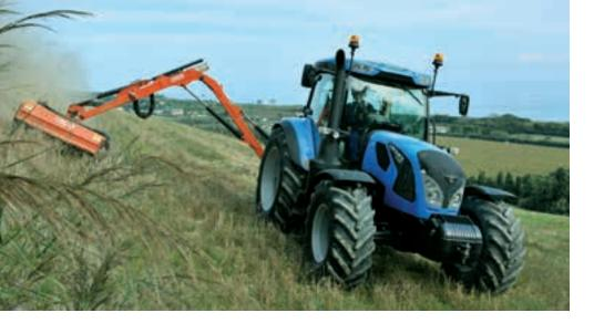
The new 6C Series from Landini is the successor to the popular Powermondial tractor family. The two models in the range are powered by the new FPT NEF 4.5L engines with power ratings of 111 hp and 121 hp.
