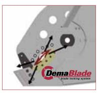
Jaw is fully guided by hardened shims. Unique, extremly robust Shear Arm Guiding System (SGS) – easy to maintain
