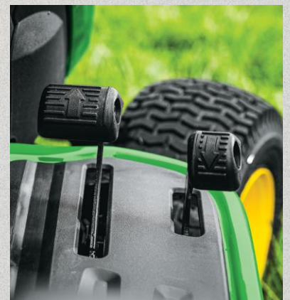
Side-by-side pedals. Easily change from forward to reverse with two-pedal foot control available on all 100 Series Lawn Tractors.
