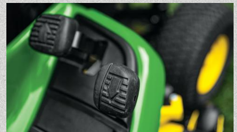
Twin Touch System. Automatic transmission lets you easily change from forward to reverse with two-pedal foot control.
