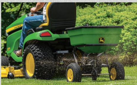
Spreader. Pull-type spin spreader available in 125lb (57 kg) or 175lb (80kg).
