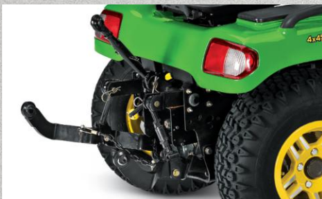
Optional Cat 0 or Cat 13-point hitch. It's the first step to tilling, cultivating and blading.
