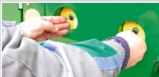
The 41 special knives which are organised in one row can be replaced and the cutting unit cleaned, without the use of tools, in approx. 5-8 minutes. Each knife is individually protected against damage from foreign objects. The cutting length of 34 mm guarantees chopping quality.
