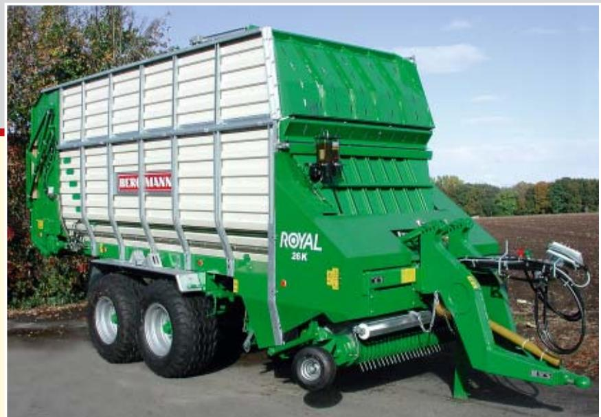
The spacious one, the Royal 26 K offers the manoeuvrability of the 24 K with a larger volume, 16 t chassis and standard DLB system. A low drawbar is optionally available. All vehicles can be equipped with 600 tires (22.5").
