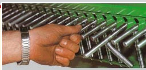
By actuating the mechanical knife pre-selection (0-41) the cut length of the material can be adapted to meet requirements. The precisely cut feed is quickly transferred to the press rotor (pre-compacting). Because of the separation of the two processes, there is no load peak. This means that crushing of the material is not possible.
