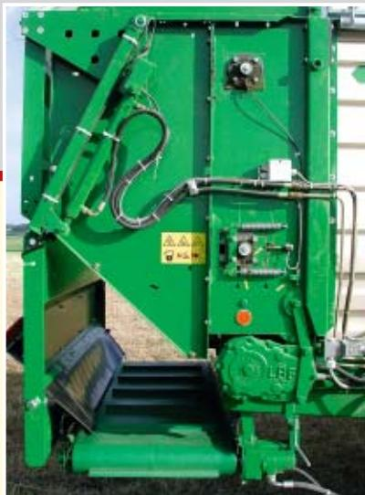
All Royal S models can be equipped with a hydraulically driven cross conveyor belt for stall feeding or filling of tower silos. When not in use, it is easily slipped under the vehicle.
