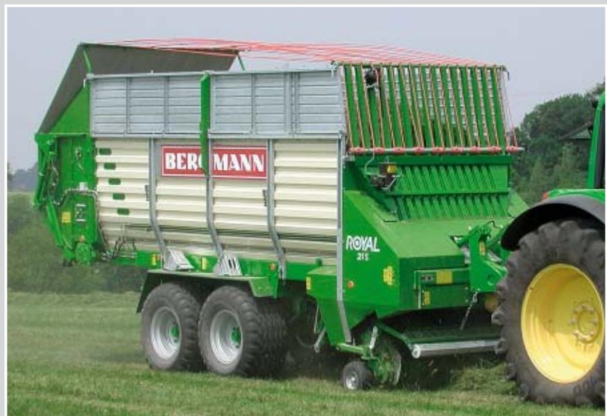
With the wind guard roller (optional) uneven swaths will be easily picked up without losses caused by wind and the pick-up (as seen here on the Royal 21S). Fold-away equipment increases the versatility.
