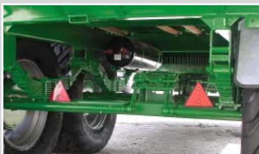
All models are equipped with a high-quality 4-spring tandem chassis. This offers high stability, driving comfort and good pulling qualities (11-16 t).
