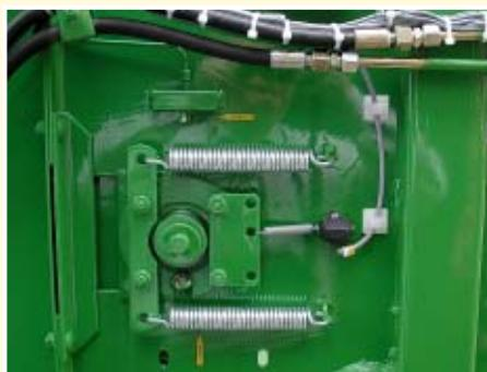
◀ The standard scraper floor control with visual level indicator provides for easy off loading.
