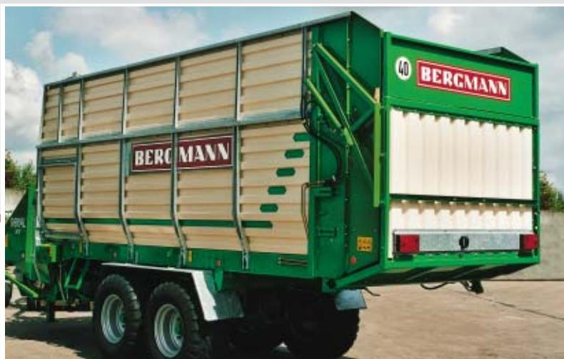
The Royal 30 K without dosing rollers combines all technical features of the S vehicle. It has a capacity of approx. 50 m<sup>3</sup> at medium compression.
