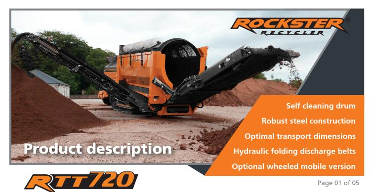
Mobile track-mounted trommel screen RTT720
