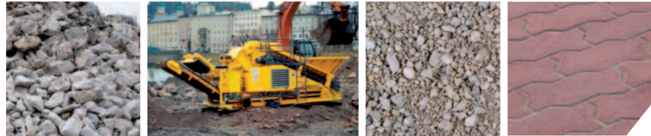
Residual concrete Processing Recycled concrete aggregate Reused as an additive in concrete production
