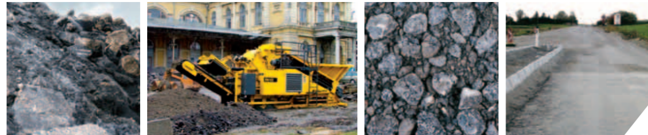
Residual asphalt Processing Recycled asphalt aggregate Reused for non-compacted load-bearing surfaces
