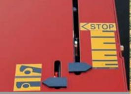
A twine arm indicator shows the progress of the wrapping cycle.
