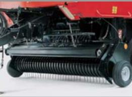
Dual flotation gauge wheels offering excellent performance in all field conditions.
