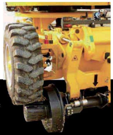
HY RAIL SYSTEM DRIVEN BY THE FOAM FILLED RUBBER ROAD WHEELS. 4X4 TRANSMISSION AND LOCKING DIFFERENTIAL. THE RAIL WHEELS HAVE A NEGATIVE BRAKING SYSTEM FOR INCREASED SAFETY. THIRD RAIL COMPLIANT.
