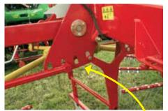
All centre swath rakes have variable working width. On the rakes you can remove the canvas and use the hole to get an even smaller working width.
