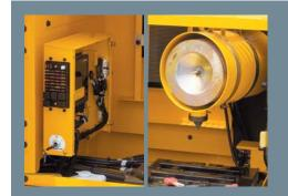
Centralized Electric Control Box and Easy Change Air Cleaner Assembly Electric control box and Air cleaner are centralized in one or the same
