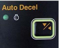
When remote-control valves are in neutral position more than 4 seconds, CPU controller instructs the accel actuator to reduce engine speed to 1100rpm. This decreases fuel consumption and reduces cab noise levels.
