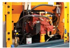
To achieve optimum precision, Hyundai redesigned the hydraulic system to provide the operator with super fine touch and improved controllability. Improved pump flow control reduces flow when controls are not being used to minimize fuel consumption.
