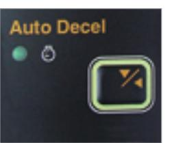
When remote-control valves are in neutral position more than 4 seconds, CPU controller instructs the accel actuator to reduce engine speed to 1,000rpm. This decreases fuel consumption and reduces cab noise levels.
