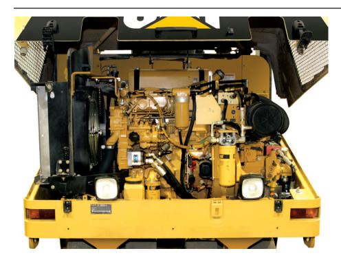
**Large engine enclosure** pivots upward for access to engine, cooling package and filters.
