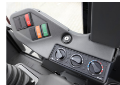
New console: ignition switch, controls for the heating and optional air-conditioning system are easy to reach
