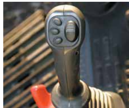
Joysticks with proportional control button for attachments
