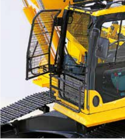
Cab front full height guard level 1 (ISO 10262)
