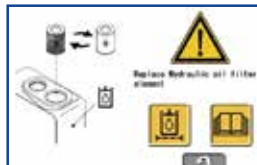
Clogging hydraulic oil filter caution
