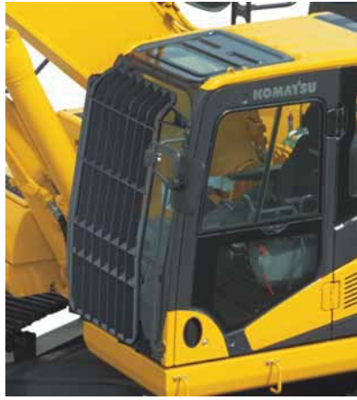
Cab front full height guard level 2 (ISO 10262)
