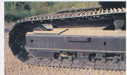
The variable gauge undercarriage gives increased stability. In addition, the track link pitch has been enlarged to the next size class, and a strut has been added for increased durability.
