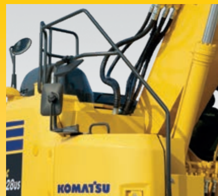
Hand rails and anti-slip plates
