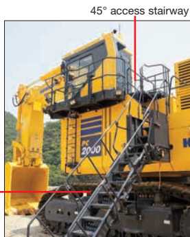
45° access hydraulically operated stairway
