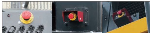
Emergency engine stop switch
