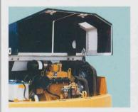
Full-open machine cover allows quick access to engine components and hydraulic equipment for quick checks and repairs. And easy air bleeding with one touch of a button.
