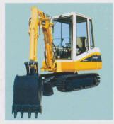
Extra-small min. swing radius and convenient boom offset enable quick dig/load operations in extra tight quarters when close to obstacles. The boom swings 50° to the left and 90° to the right. In addition, the PC20-6 attains a wide working range. Reinforced dozer blade with cutting edge is ideal for refilling and leveling.
