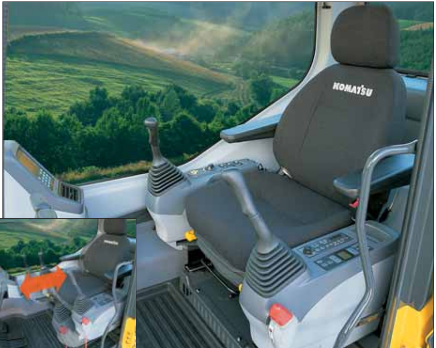
Seat Sliding Amount: 340 mm 13.4", increased 120 mm 4.7"
