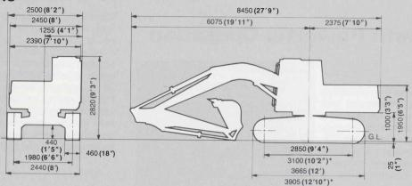
With 5150 mm (16'11") one-piece boom, 2610 mm (8'7") arm, SAE heaped 0.63 m<sup>3</sup> (0.82 yd<sup>3</sup>) backhoe bucket. \*LC undercarriage dimensions
