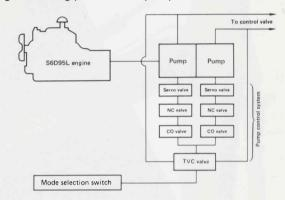
**OLSS (Open-Center Load Sensing System)** — is built into the hydraulic system as a means of reducing unnecessary hydraulic losses.
