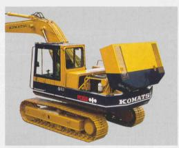
**Travel motors** — are always protected from external damage since they are in-shoe type motors. Also, all hydraulic piping is safely routed through the rolled box X-leg center frame.
