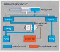
When only the arm is actuated oil flow from two pumps is merged and sent to the arm circuit, accelerating arm speed.
