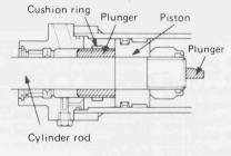
**Straight travel valve** — automatically interlocks the left and right hydraulic circuits allowing the machine to always travel straight, even when work equipment is being simultaneously operated.
