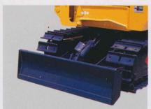
**Dozer blade:** This toughly constructed blade is ideal for refilling and leveling. Due to the advanced control valve mechanism, simultaneous blade actions and machine travel are smooth.
