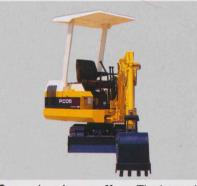
Convenient boom offset: The boom itself can be swung 50° to left and 70° (or 90° as an option) to right side. This means that the PC05-6 can complete quick dig/load operations in extra tight quarters without swinging the upper structure of which the tail end may hit obstacles such as walls, poles, etc.
