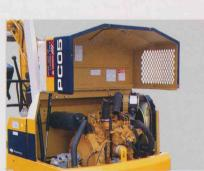
Full-open machine cover allows quick access to internal components such as engine, hydraulic equipment, etc. for both quick checking and repairing.
