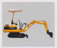
Wide working range: Equipped with the long boom and arm, the PC05-6 attains a wide working range. This, plus large breakout force make it easy to conduct any type of excavation work.
